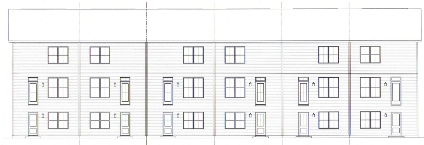
2 6-UNIT BUILDING REAR ELEVATION A-2.2 SCALE: 3/16" = 1'-0" 3-STORY PLAN
