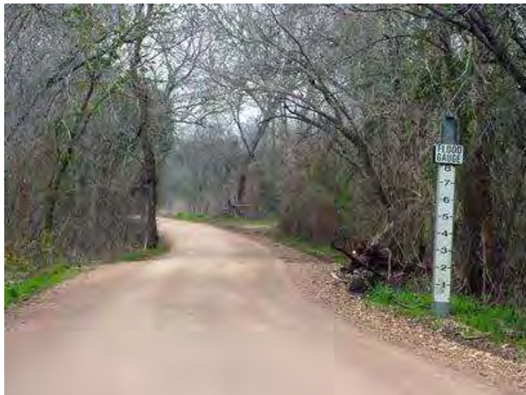
Figure 20: Example of a Roadside Flood Gauge Source: Google
